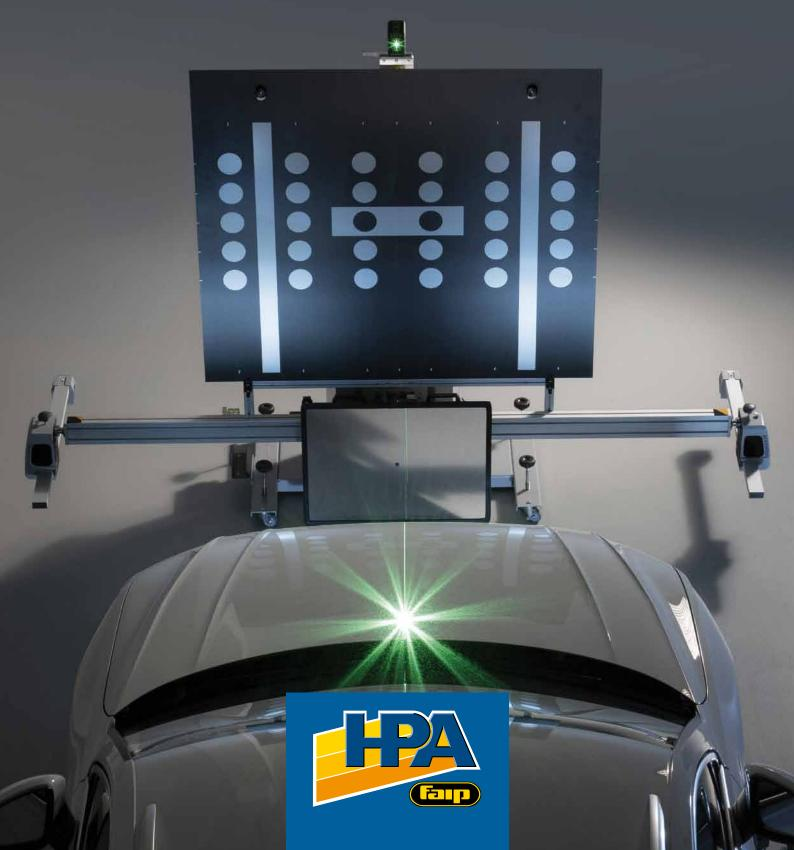
**PROADAS** is the universal modular system developed for check and **calibration of driver assistance systems** (front sensors), **check of the alignment status** and **complete wheel alignment service** (optional) on multi-brand vehicles and commercial vehicles.
